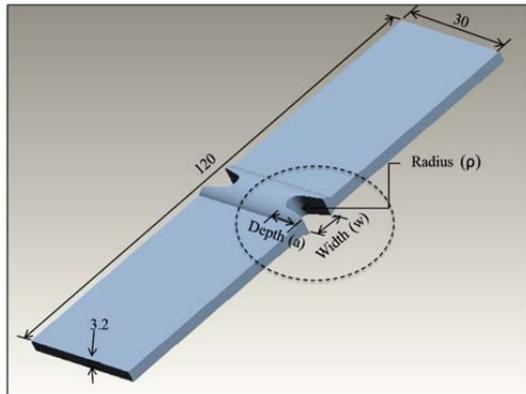
Fig. 2: Geometry of Welded Double Edge Notched Tensile (DENT) specimen (all dimensions are in mm).
