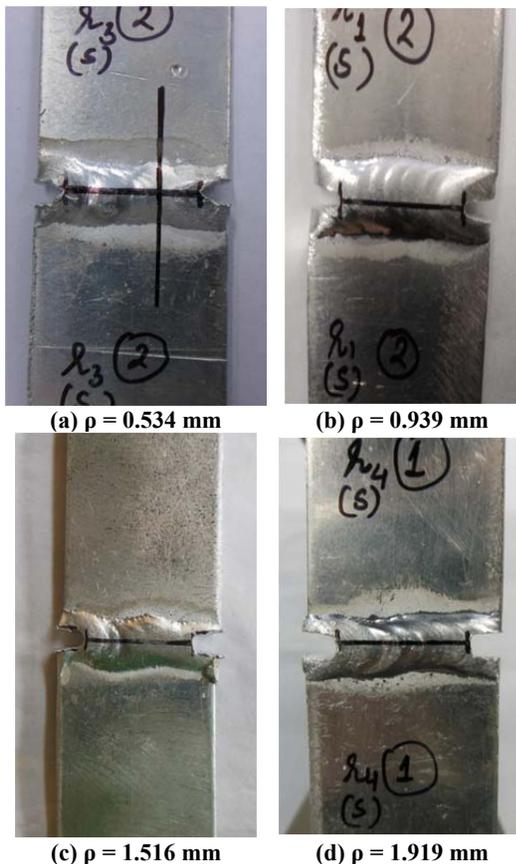
Fig. 3: Images of Welded Double Edge Notched Tensile (DENT) specimens with different notch radius.
